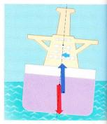
When a ship tilts, the buoyant force shifts; buoyancy's upward push and gravity's downward pull right the ship.
