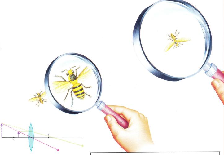
When an object (solid arrow) is closer to the lens than the focal point (F) is, the lens creates a virtual image (purple dashes) that is the right way up and magnified.
