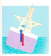
If a tilting ship's centre of gravity moves too high and lies too far from the centre of buoyancy, the ship will capsize.
