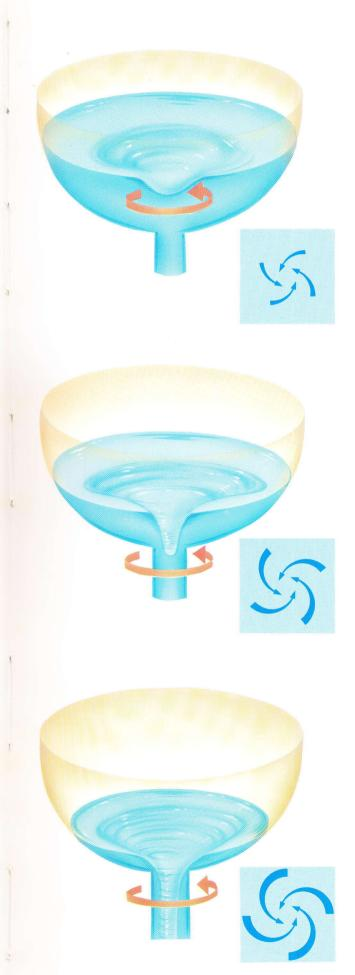
2 Once the water starts to move in a circular path, other water molecules follow. The closer the particles are to the drain, the faster they move. Those farthest from the centre travel most slowly.
