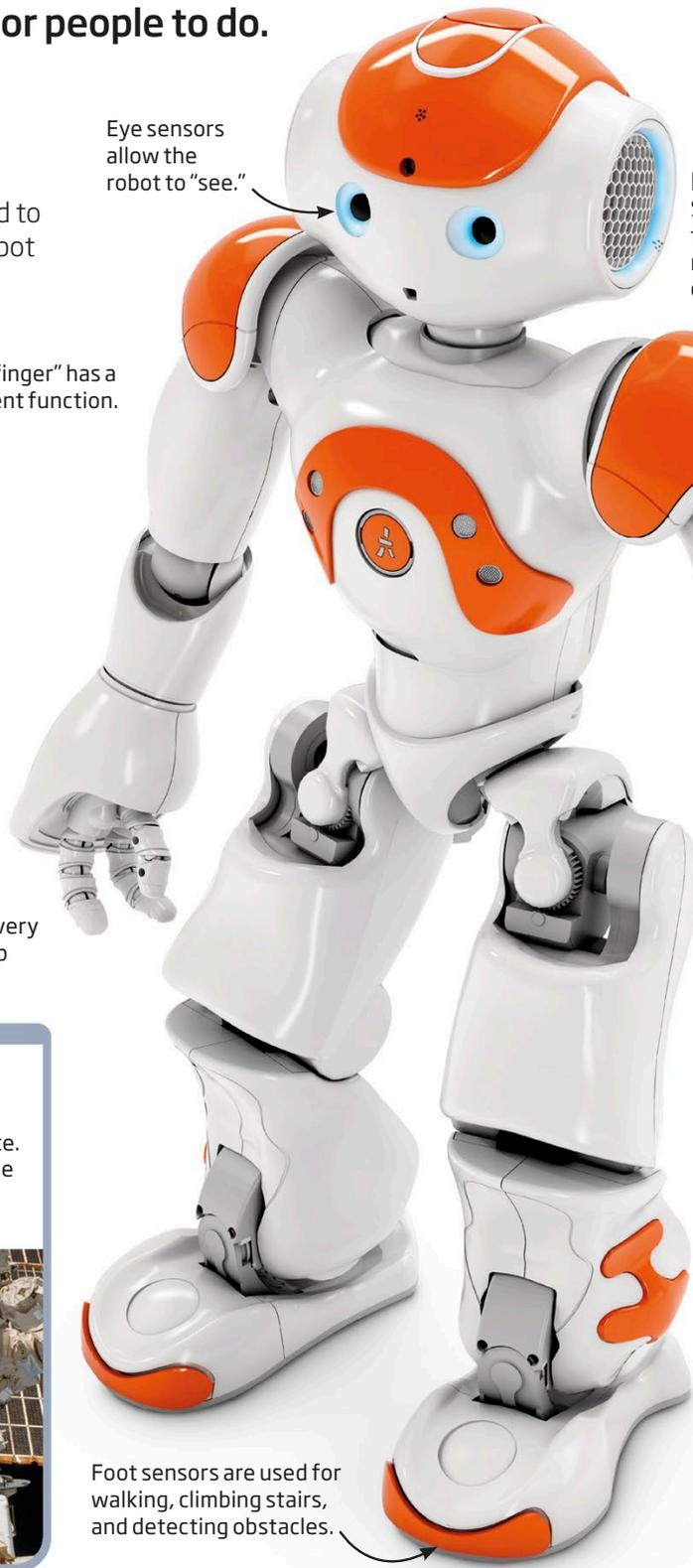
Eye sensors allow the robot to "see."
